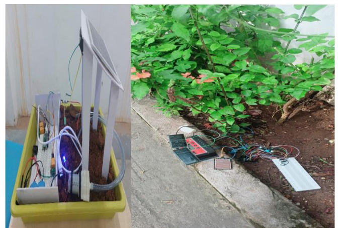
Figure 3 Experimental Setup for IOT Enabled Remote Control Smart Garden with Solar System
