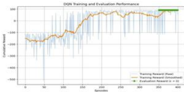
Figure 1 Training and evaluation performance of the Proposed Deep Q-Network (DQN) Model. The Raw Cumulative Reward Curve Illustrates Exploration Induced Variance During Training, While The Moving-Average Smoothed Curve Highlights Stable Convergence.
