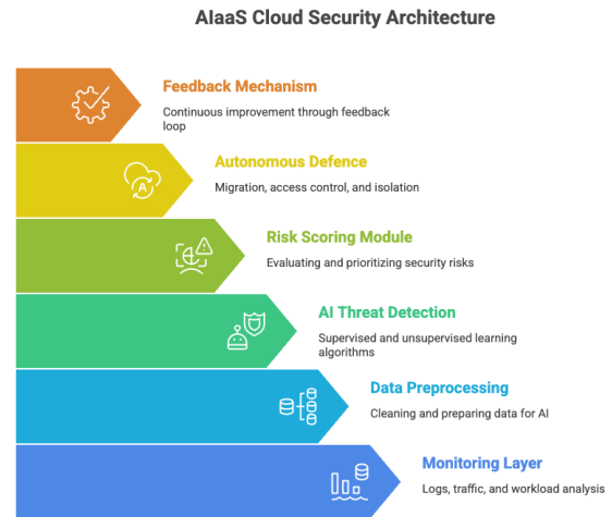
Figure 1 AIaaS Cloud Security Architecture
