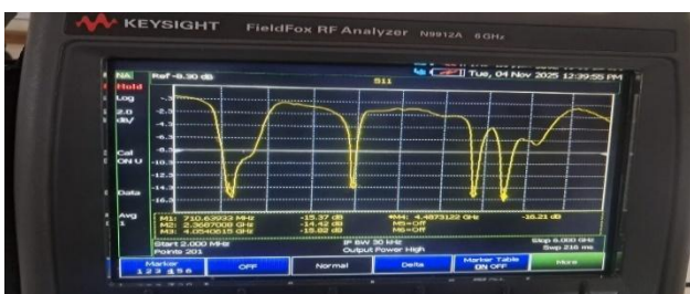
Figure 6. Measured s11 using analyzer
