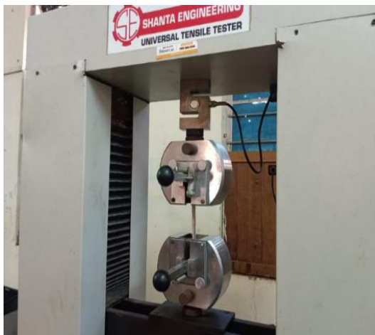
Figure 3 Experimental Setup for Tensile Strength Analysis
