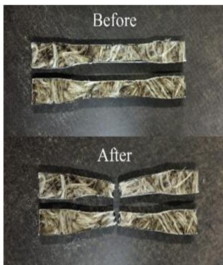
Figure 4 Specimen Condition Before and After Tensile Testing
