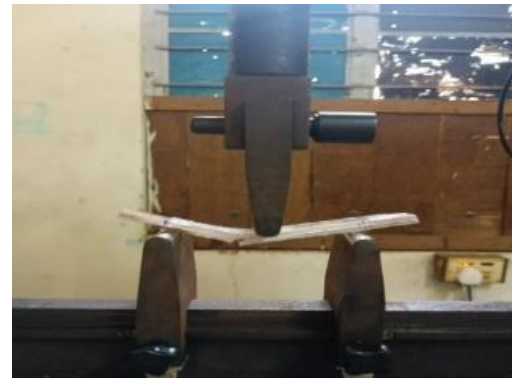
Figure 5 Flexural Strength Measurement Using UTM
