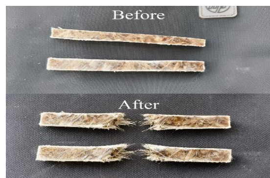
Figure 6 Specimen Appearance Before and After Flexural Testing
