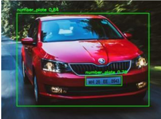
Figure 2 License Plate Recognition (LPR) using YOLOv8
