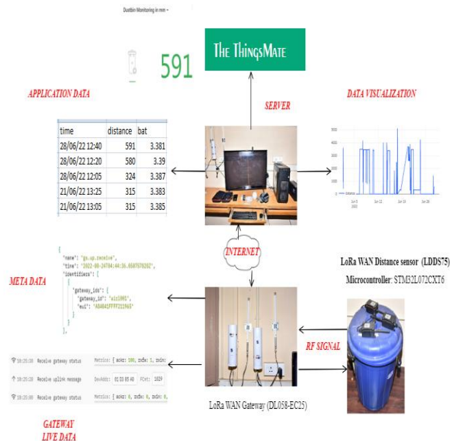
Figure 6 Experimental setup of a LoRa WAN ultrasonic sensor
