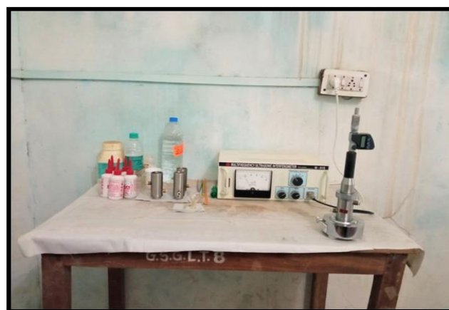
Figure 2 Experimental Arrangement for Multi-Frequency Ultrasonic Device
