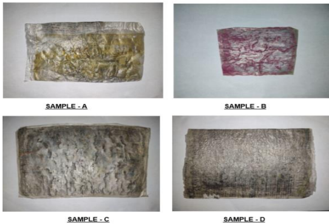
Figure 4 Various Samples Prepared According to the Number of Layers of Carry Bags
