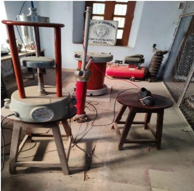
Figure 5 Experimental Setup of HV Testing
