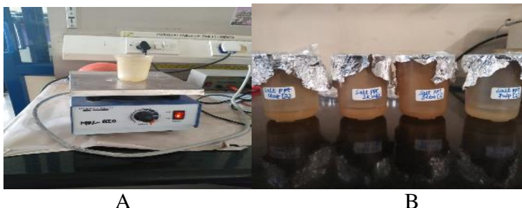
Figure 3 A. Ammonium Salt Precipitation Using A Stirrer. B. Ammonium Sulphate Extraction
