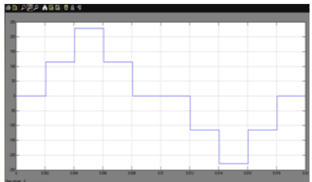
Figure 27 Output Voltage of Five-level Multi Modular Inverter without Filter
