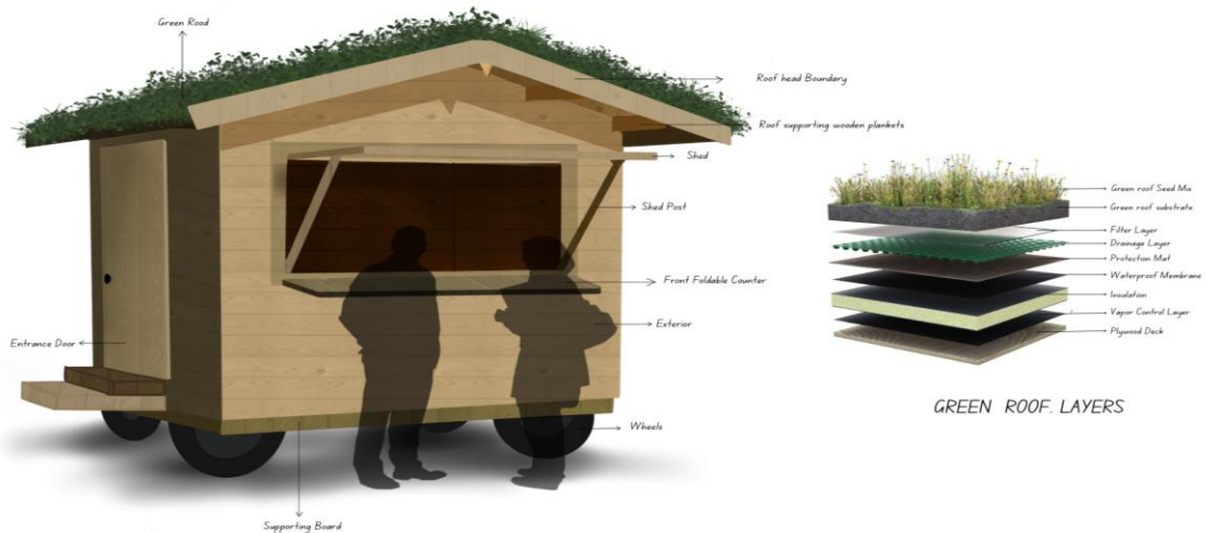
Figure 8 Integration of Green Roof
