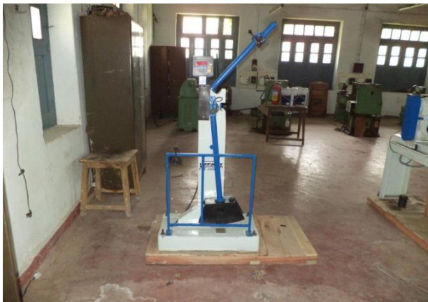
Figure 3 Impact Testing Machine
