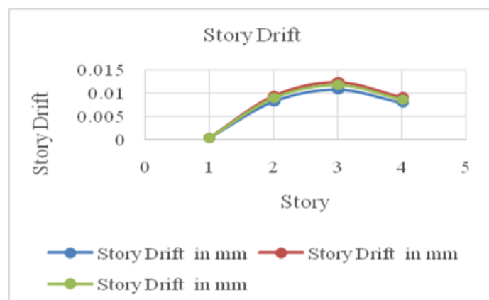
Figure 23 Story Drift with Comparison of Different Bracing
