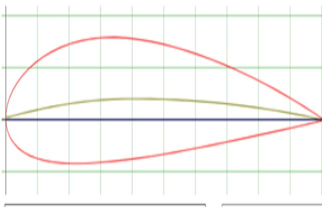
Figure 1 NACA-2421 Airfoil [1]
