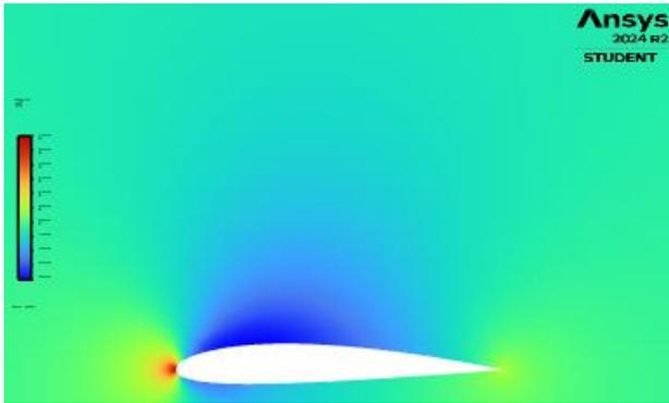
Figure 5(a) Pressure Contour(Magnified)
