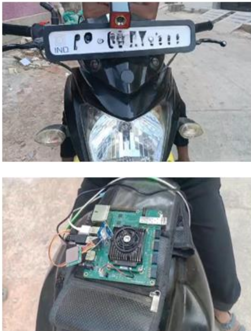
Figure 4 Front View and Placement of the Vehicle-Mounted Deployment Setup
